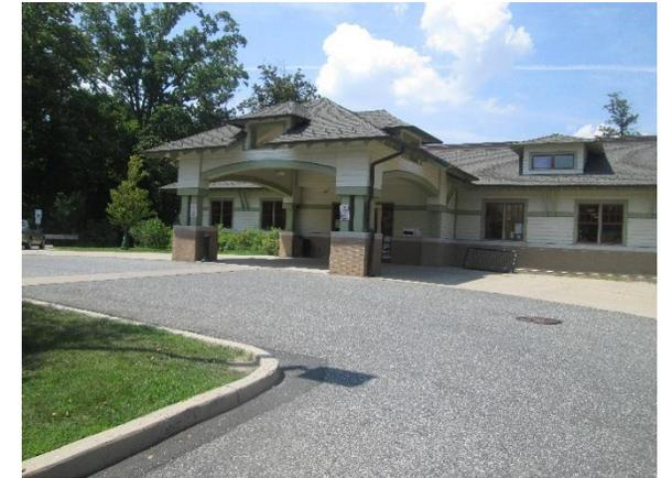
Selected sections of parking can be replaced with porous asphalt to capture and infiltrate stormwater generated by the parking lot. A rain garden can be installed off of the northwest corner of the building to capture, treat, and infiltrate roof runoff. A preliminary soil assessment suggests that the soils have suitable drainage characteristics for green infrastructure.
