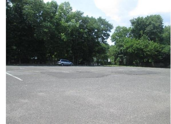
The parking lot was in poor condition at the time of the assessment. Multiple rows of parking can be replaced with porous asphalt to capture and infiltrate stormwater. A preliminary soil assessment suggests that the soils have suitable drainage characteristics for green infrastructure.
