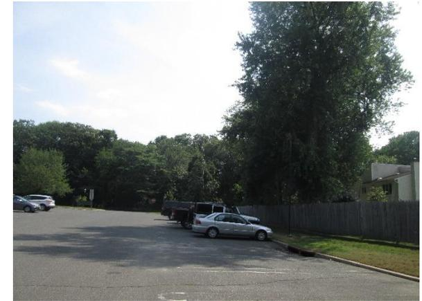
Multiple rows of parking can be replaced with porous asphalt to capture and infiltrate stormwater. On the south side of the building a rain garden can be installed and two downspouts can be disconnected and redirected into it to capture, treat, and infiltrate roof runoff. A preliminary soil assessment suggests that the soils have suitable drainage characteristics for green infrastructure.
