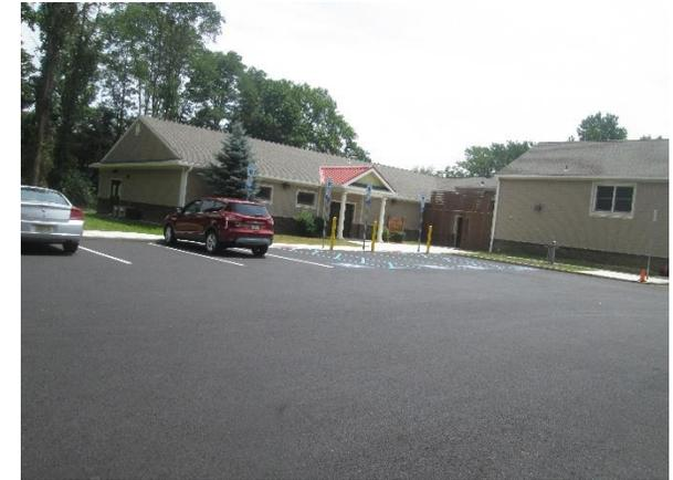
Sections of the parking lot can be replaced with porous asphalt to capture and infiltrate stormwater. A rain garden can be built off of the southwest corner of the building to capture, treat, and infiltrate roof runoff. A preliminary soil assessment suggests that more soil testing would be required before determining the soil's suitability for green infrastructure.
